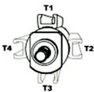
View from front (rod end) with front and rear ports aligned along position T1
